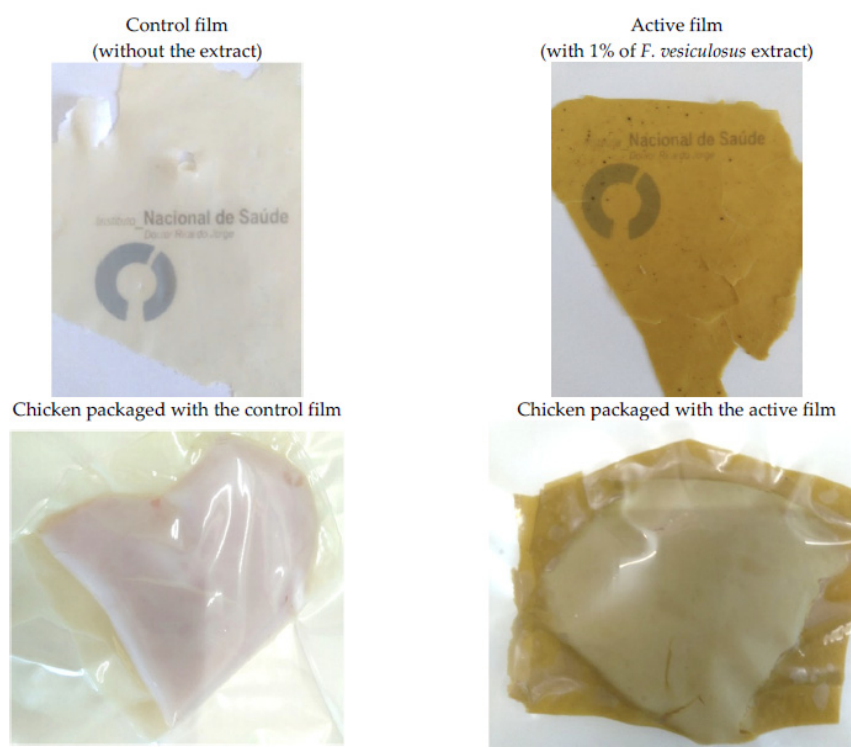
Figure 2. Whey protein control film and active film with 1% Fucus vesiculosus (brown seaweed) extract [29].
