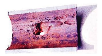
Figure 2.4. Deep, round, and elongated pits at the internal surface of tubing [9].
