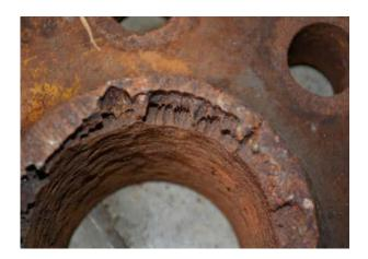
Figure 2.5. Changeover 3 in. × 6 in. diameter, gas producer with 4.5% CO<sub>2</sub>, erosion–corrosion damage on the 3 in. side [9].
