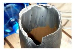
Figure 2.6. SCC attack on a pipeline section [10].
