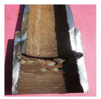
Figure 2.2. Selective attack on the internal surface at the thread juncture of the tubing and the tubing box [6].
