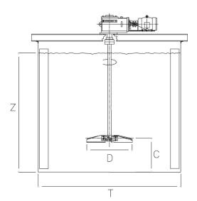
In addition to maintaining geometric similarity, the same impeller style should be used throughout the scale-up process.
