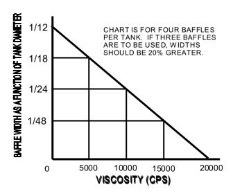
The reason for a decreasing need for baffles, as the viscosity increases, is that high viscosity liquids offer fluid flow resistance which produces less swirl and more vertical flow for the same power input as equal amounts of low viscosity liquids.
