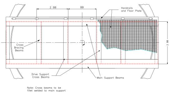
Note: Cross beams to be fillet welded to main support beams completely around each joint.
