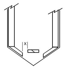
Deep dished (spherical) tanks should have baffles extend into the bottom head to ensure good mixing results in this region. In addition, if low level mixing is required in a semi-elliptical head these tanks should also have the baffles extend into the lower head. Ideally, the baffle shape should conform to head profile, however, straight baffles have been used with acceptable results. The baffle in this portion of the tank should have the same geometry as for a cone bottom tank.
