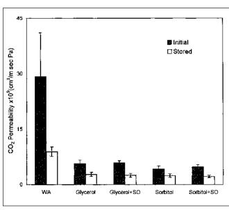
Fig. 1–Effect of storage time (20 d at 20 °C and 63.8% relative humidity) on  $CO_2$  permeability of corn starch-based films. WA: without additives, SO: sunflower oil (2g/L), plasticizer concentration (glycerol or sorbitol): 20g/L
