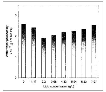
Fig. 2—Effect of lipid concentration (sunflower oil) on water vapor permeability of corn starch films plasticized with 20g/L glycerol. Maximum standard deviation = 0.53
