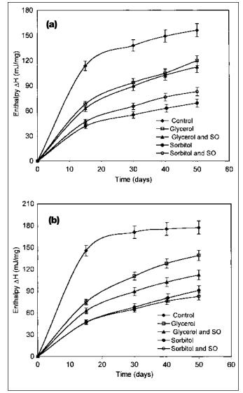
Fig. 3–Effect of plasticizer and lipid presence on transition enthalpy of (a) corn starch films and (b) amylomaize films stored at 20 °C and 63.8 % relative humidity. ( $\blacklozenge$ )Control films without plasticizer, ( $\square$ ) films with 20g/L glycerol, ( $\blacktriangle$ ) films with 20g/L glycerol and 2g/L sunflower oil, ( $\blacklozenge$ ) films with 20g/L sorbitol, ( $\bigcirc$ ) films with 20g/L sorbitol and 2g/L of sunflower oil
