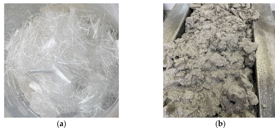
Figure 2. Polypropylene fibers (a) as received; (b) during mixing.
