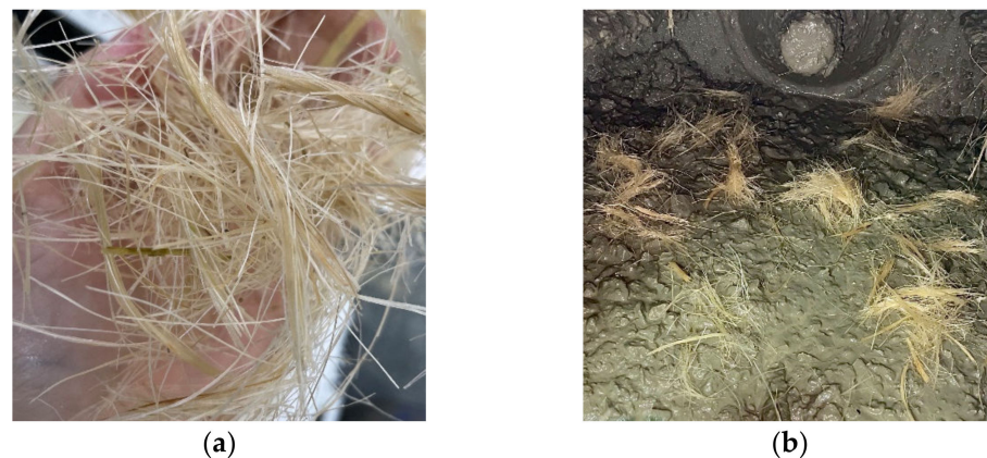
Figure 1. Sisal fibers (a) as received; (b) cut to length during mixing.
