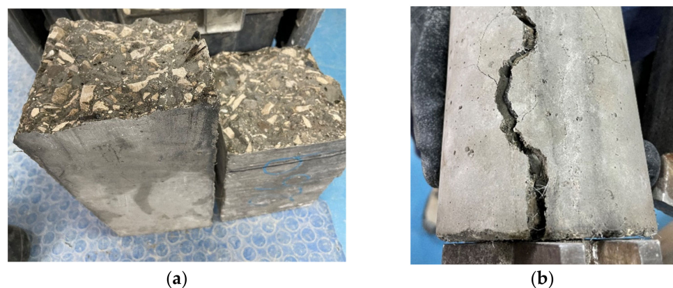
Figure 7. (a) Beam tested in flexure after failure; (b) Splitting tensile strength tested cylinder after load.
