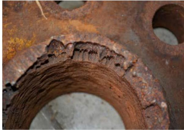
Figure 2.5. Changeover 3 in.  $\times$  6 in. diameter, gas producer with 4.5% CO<sub>2</sub>, erosion–corrosion damage on the 3 in. side [9].
