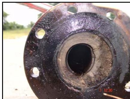
Figure 9. State of the wellhead of the selected well before the field test
