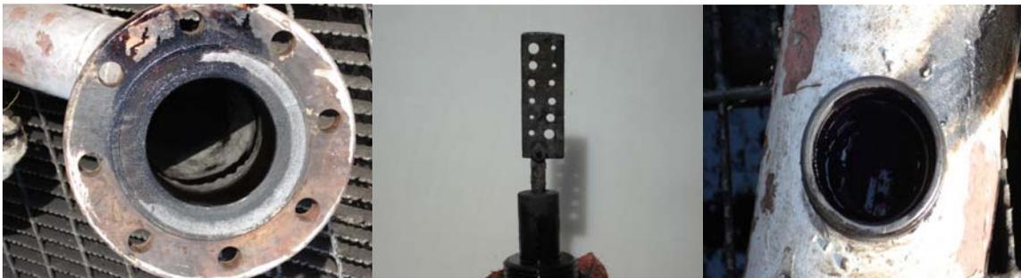
Figure 12. State of the wellhead, coupon and couponholder of the selected well at 20 days since the start of the field test at 20 days after the start of the field test
