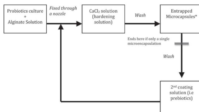
**Fig 2:** Flow diagram of extrusion process. The bacterial culture with alginate is dropped using a nozzle into hardening solution. The produced microcapsules are added into a second coating solution, if required. The process ends at \* if only a single encapsulation is required (Krasaekoopt *et al.*, 2003).
