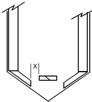
Deep dished (spherical) tanks should have baffles extend into the bottom head to ensure good mixing results in this region. In addition, if low level mixing is required in a semi-elliptical head these tanks should also have the baffles extend into the lower head. Ideally, the baffle shape should conform to head profile, however, straight baffles have been used with acceptable results. The baffle in this portion of the tank should have the same geometry as for a cone bottom tank.
