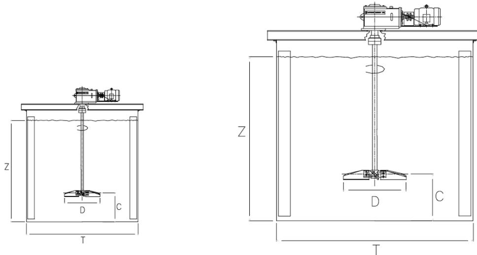
In addition to maintaining geometric similarity, the same impeller style should be used throughout the scale-up process.
