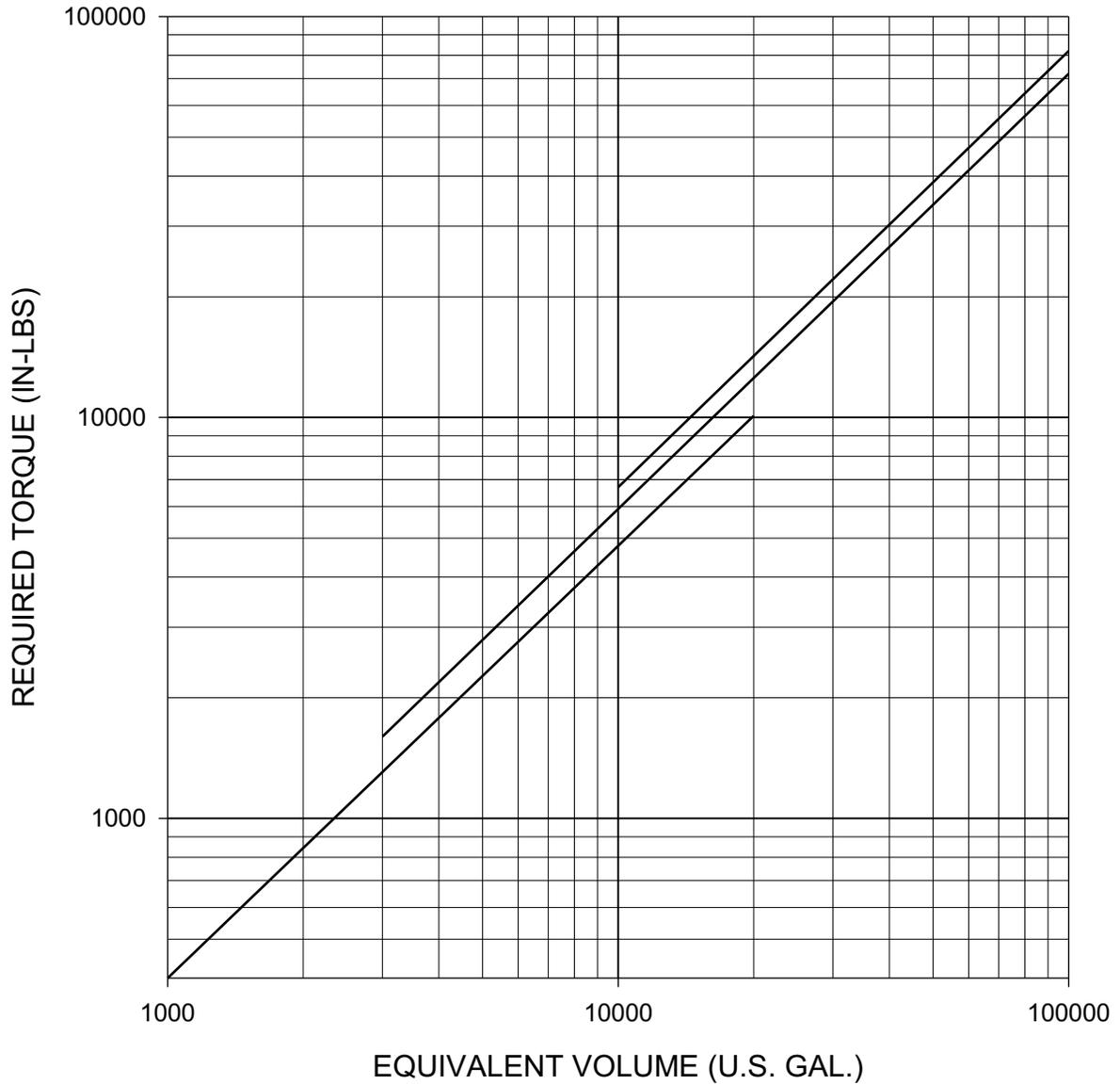
**FREE SETTLING SOLIDS SUSPENSION APPLICATIONS**
