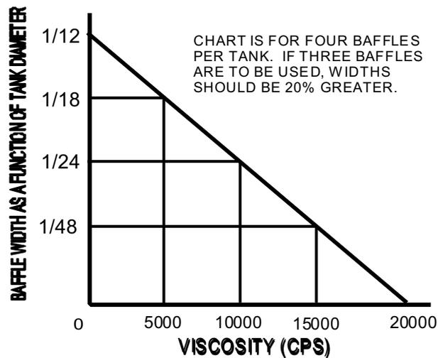
The reason for a decreasing need for baffles, as the viscosity increases, is that high viscosity liquids offer fluid flow resistance which produces less swirl and more vertical flow for the same power input as equal amounts of low viscosity liquids.
