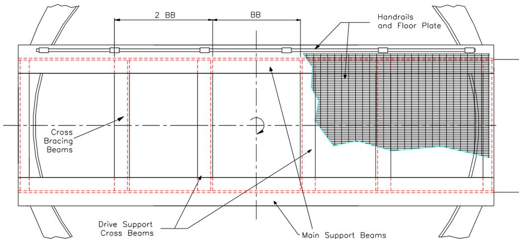
Note: Cross beams to be fillet welded to main support beams completely around each joint.
