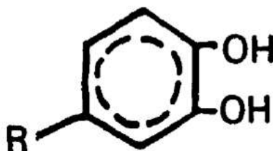
Fig. (2-2): Pyrocatechol forms insoluble chelate complex with the metal, efficient corrosion inhibitor [41].
