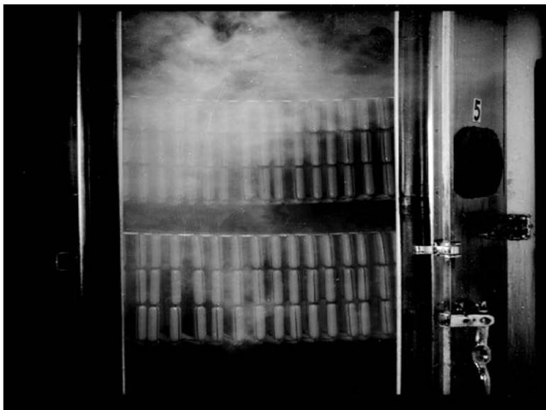
**Fig. 10.6** Atomization cloud in a smokehouse (courtesy of Red Arrow Products Company LLC, Manitowoc, Wisconsin, USA).
